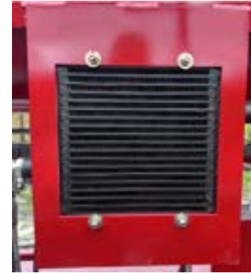
Hydraulic Oil Cooler
