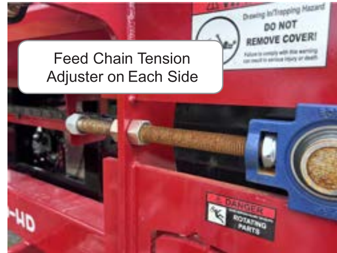
Feed Trough Chain Tension Set Screw
